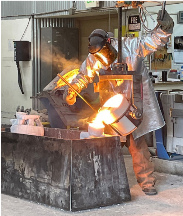
Pouring molten bronze into a ceramic shell.
