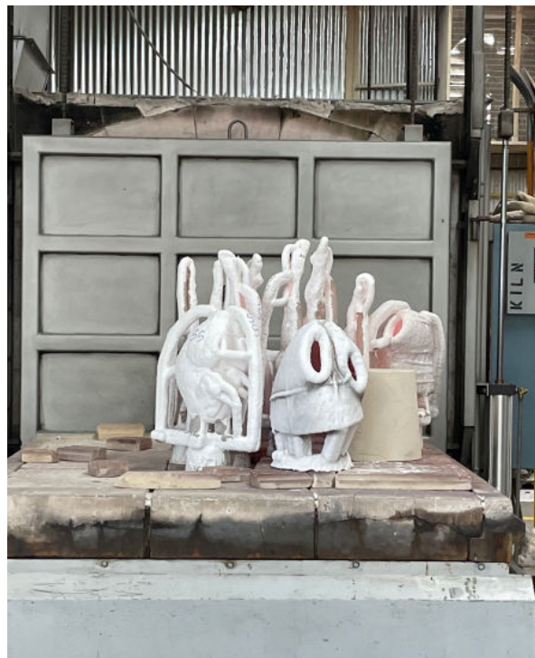
Ceramic Shells coming out of the kiln
